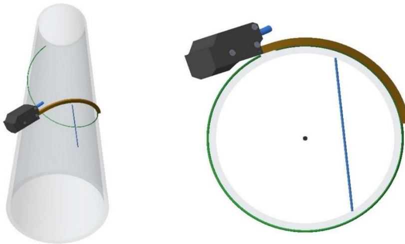
Figure 3: Xsens helical signal excitation and chordal signal transmission
